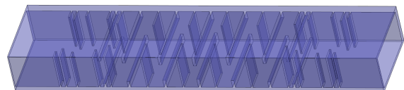
图 13 接收频段带通滤波器结构示意图 Fig. 13 Schematic diagram of band-pass filter structure in receiving band
