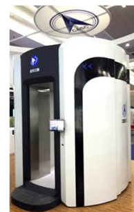
图 3 北遥所太赫兹人体安检仪样机 Fig. 3 Demonstration of THz body security apparatus by BRIT
